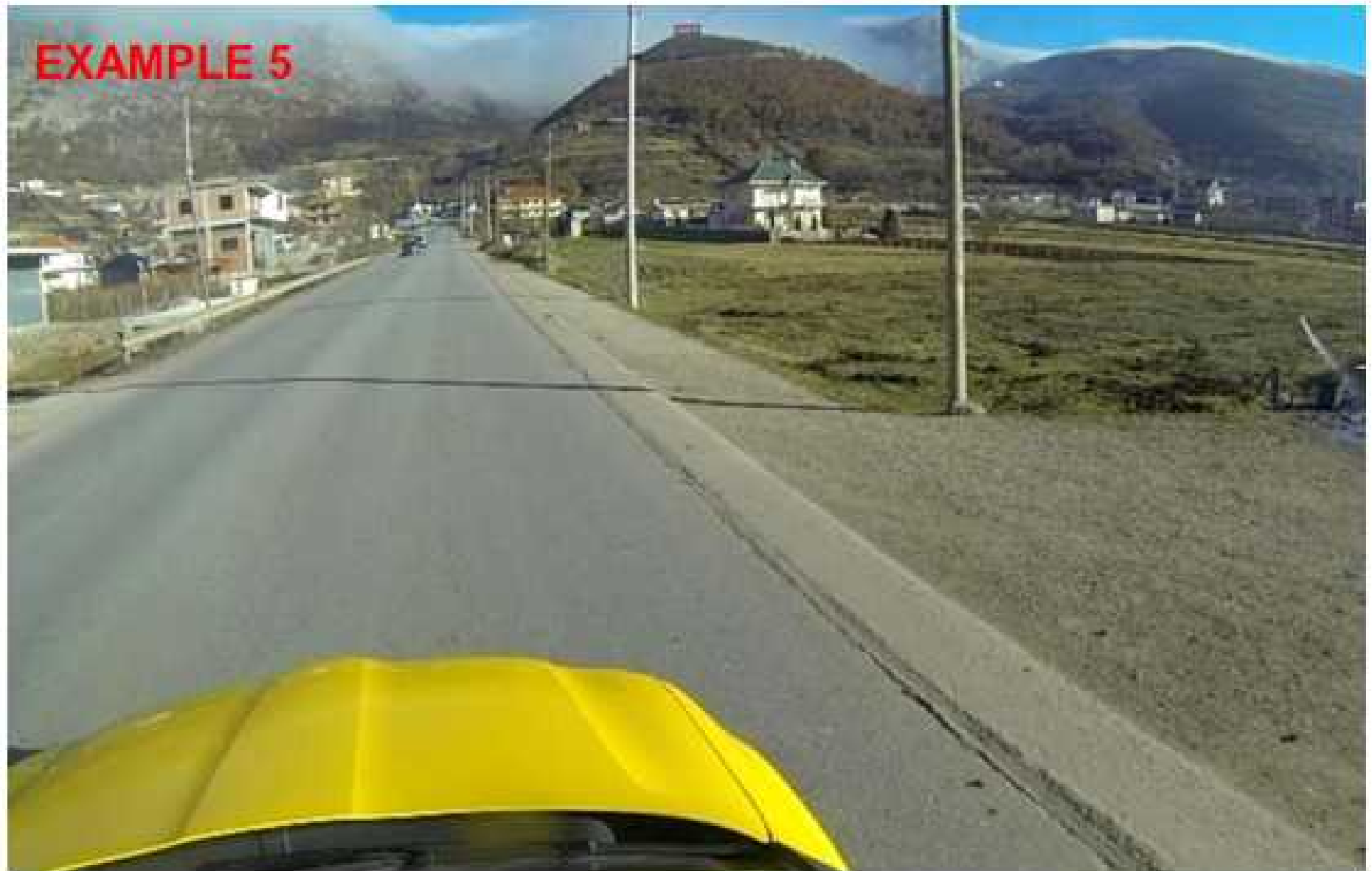
Example 5 – Poles and posts are common type of hazardous objects on the roadside.
